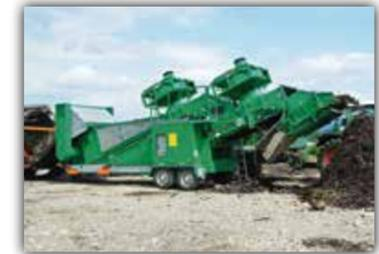
Specifically built to separate plastic, the Hurrikan S mobile high-throughput windsifters remove light fraction plastics, rocks using a patented "pressure-suction" process.
