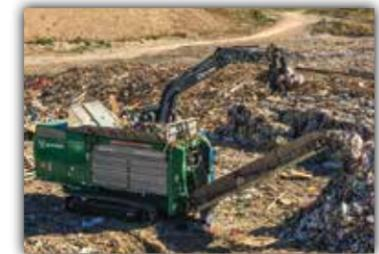
A low-speed, high-torque single shaft shredder, the Terminator processes all types of waste including contaminated C & D debris, bulky waste, mattresses, tires, and municipal solid waste.
