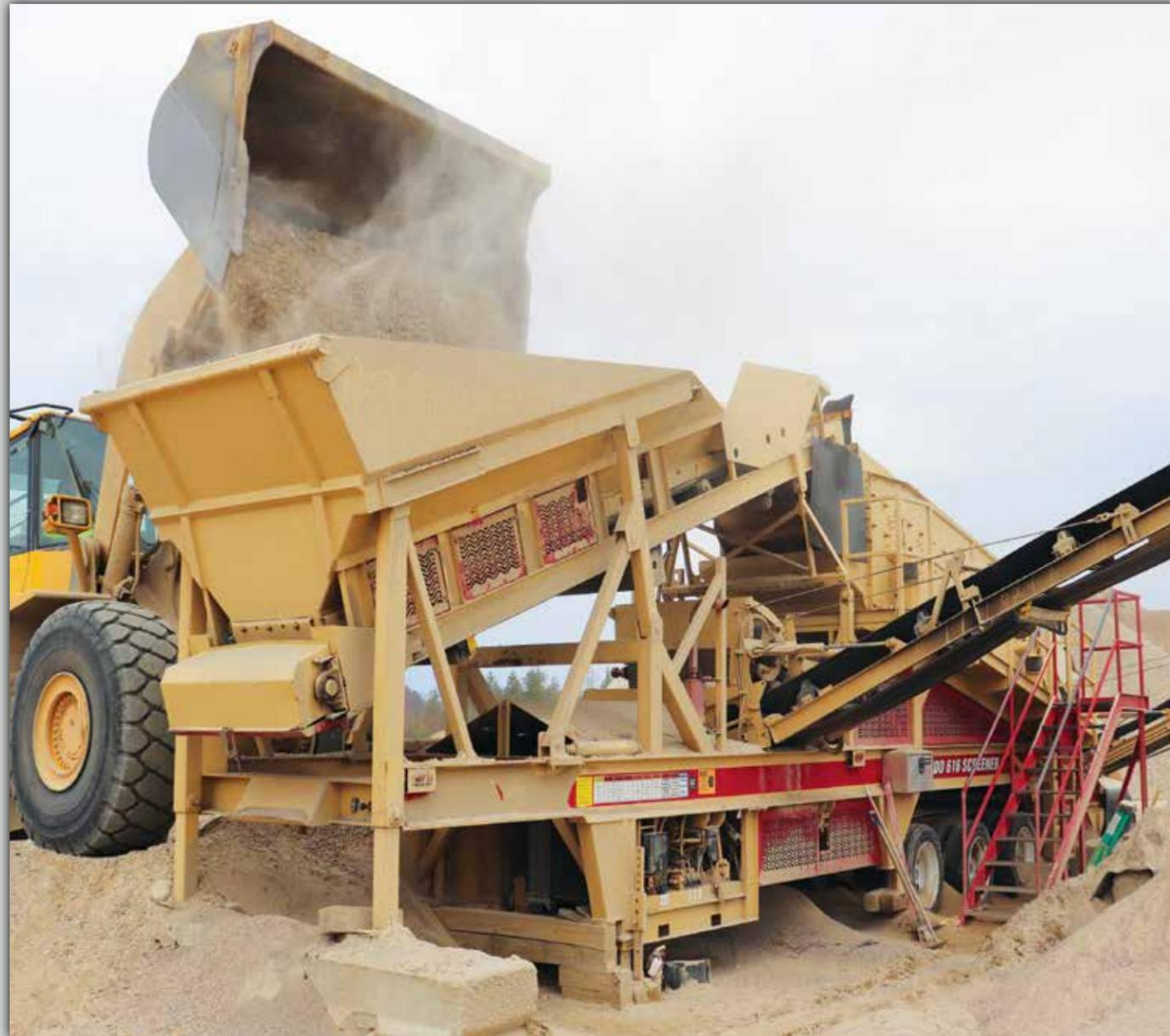
Tough as the materials it screens, the RDO 616 screener is available in 2- or 3-deck models and thoroughly sorts rock, stone, concrete, and sand.
