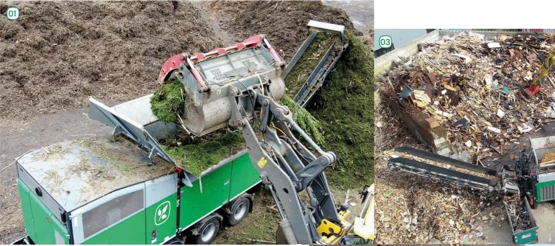
A high throughput of bulky vegetation is made possible by the generously dimensioned feed area, folding hopper and counter-rotating teeth. Blockages from wet material and high grass content are practically impossible. The teeth clear the screen baskets on every revolution.
