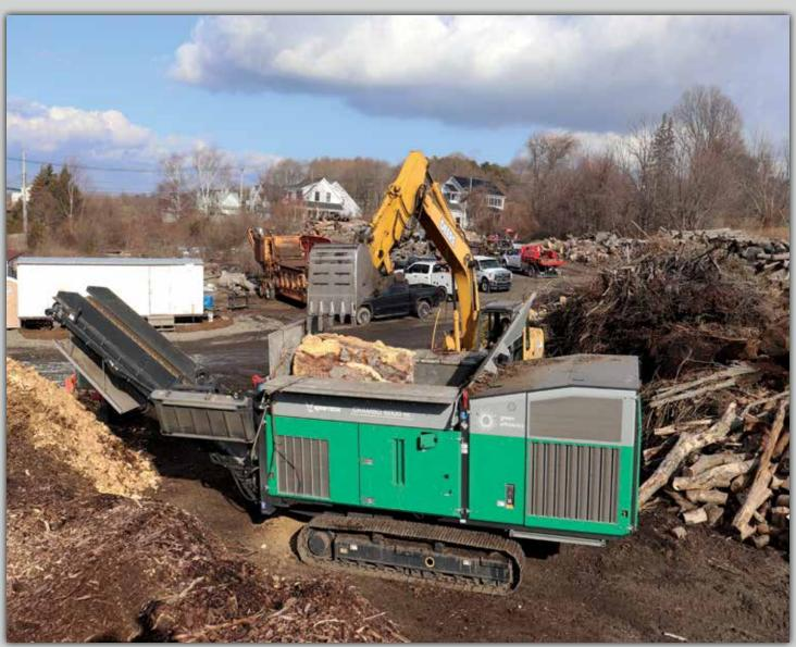
Komptech's Crambo is a low-speed, dual-shaft shredder engineered to deliver high-throughput shredding for wood and organic waste.
