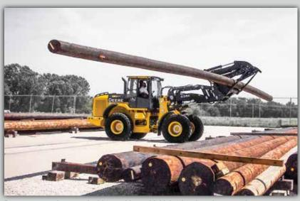
Dymax accessories are suited for machines with higher breakout forces, and are designed to match individual loader characteristics, typically yielding additional capacity and production.
