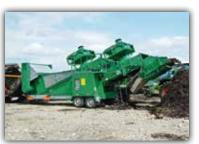
Specifically built to separate plastic, the Hurrikan S mobile high-throughput windsifters remove light fraction plastics, rocks using a patented "pressure-suction" process.
