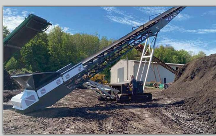
The MGL 842 T is an 80' tracked stacker with a conveyor that has a 42" wide smooth belt, a reversing fan, and a fuel-efficient motor
